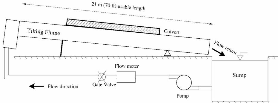
Fig. 2 Flume schematic (not to scale)
