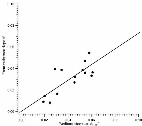
Fig. 8 Form resistance slope vs. bedform steepness
