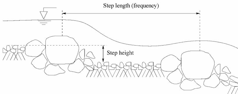
**Fig. 1b** Schematic of step-pool configuration
