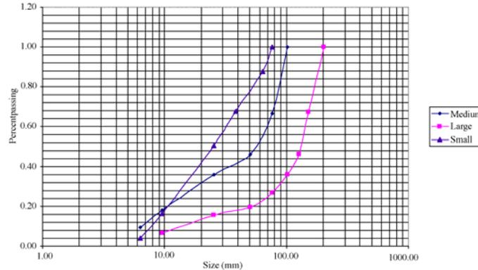
Fig. 3 Sediment size distributions tested
