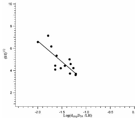
**Fig. 7** Friction factor regression analysis
