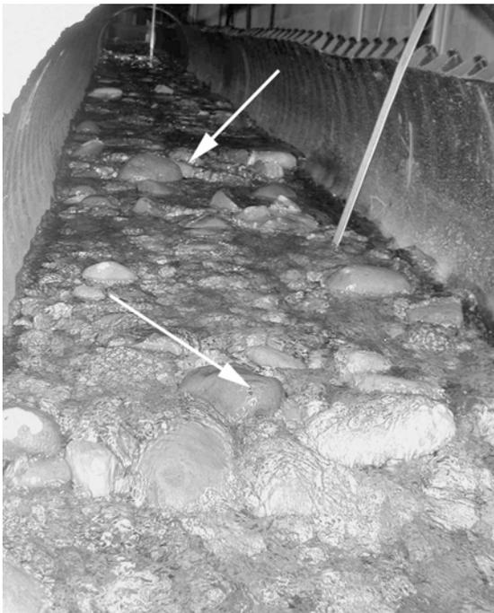
**Fig. 4a** Typical step-pool formation at 5% slope
